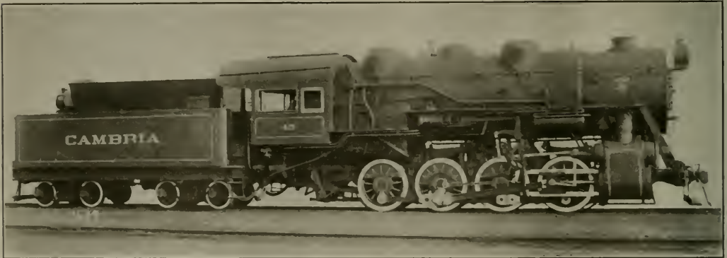
EIGHT-COUPLED SWITCHER TYPE LOCOMOTIVE FOR THE CAMBRIA STEEL COMPANY. Baldwin Locomotive Works, Builders.
